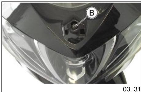
Unscrew and remove the front screw «B».
