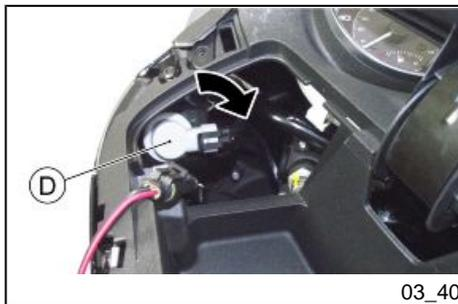
Turn the lamp holder «D» by 1/4 a turn clockwise and remove it.
