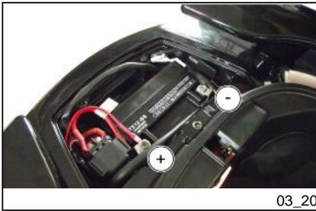
The battery is the electrical device that requires the most frequent attention and the most thorough maintenance.
