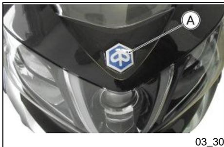
Using a screwdriver and paying attention to the bodywork, remove the Piaggio clip-on badge «A».
