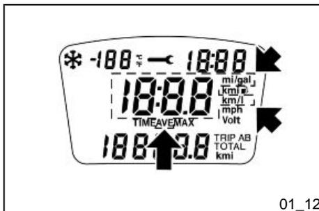
The travel is displayed only if the speed is greater than 5 km/h (3 mph), otherwise the symbol «--.» is displayed.
